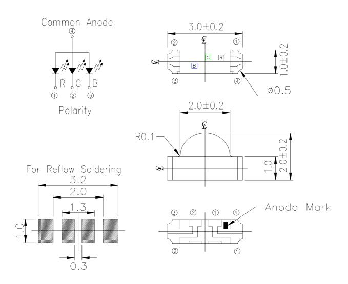
**Note:** The tolerances unless mentioned is  $\pm 0.1$ mm, Angle $\pm 0.5^{\circ}$ , Unit = mm
