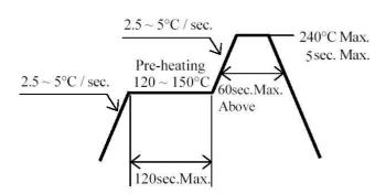
3.2 Lead free solder Lead solder temperature profile
